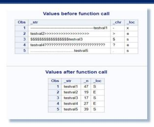
PROC FCMP provides the special function named RUN\_MACRO that enables a user-written routine to run a macro. There is no restriction as to what the macro can generate in terms of SAS code: it can include a number of DATA steps and PROC steps. Since a user-written routine is callable from within a DATA step then RUN\_MACRO makes it's possible to have nested DATA steps. References by Carpenter (2016) and Deguire (2013) provide more detail on the use of RUN\_MACRO.
