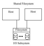
The shared filesystem solution (NAS) scales to multiple hosts in a simple fashion that introduces very little overhead due to the additional hosts.
